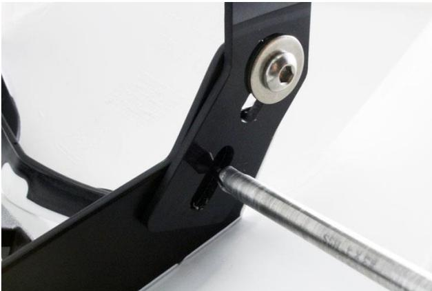
2. Using a 1/4" drill bit, drill out the bottom hole through stock headlight shell.
