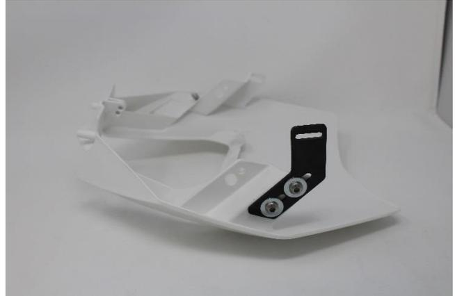
5. Slide the light into the housing lining it up the ears to bolt hole in the bezel. Put the spacer in between the ear and the light bezel. Insert the M6X40 with the washer from the front of the light, through the spacer and the ear, install the M4 nut. **NOTE:** Do not over tighten, you may risk cracking the plastic ear on the mask.
