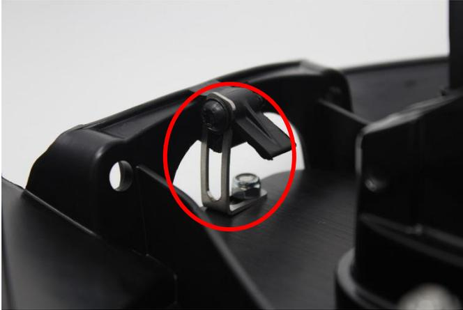
7. Using the provided black screw, install it in the hole that is closer to the back of the bike. To obtain full downward adjustment, you must trim the hole furthest from the chassis to allow the nyloc nut to clear. (Refer to circled area in figure 6)
